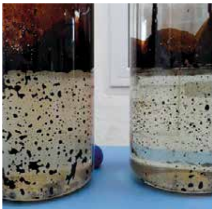
JARTEST for oil/water separation test before disposal into the sea
